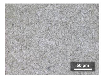
Microstructure after heat treatment at  $500^{\circ}\text{C/2h} + 1075^{\circ}\text{C/30min} + \text{Cryogenic treatment at } -80^{\circ}\text{C} + 2 \times 525^{\circ}\text{C/2h}$  for a hardness of 56 HRC.
