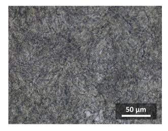
Microstructure after heat treatment at  $500^{\circ}\text{C/2h}$  +Cryogenic treatment at - $80^{\circ}\text{C}$  + 2 x  $550^{\circ}\text{C/2h}$  for a hardness of 53.6 HRC.
