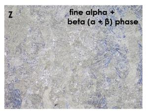
Microstructure for Stellar Ti6Al4V ELI obtained after Kroll etching.
