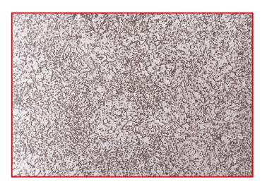
STRUCTURE IN THE ANNEALED CONDITION
