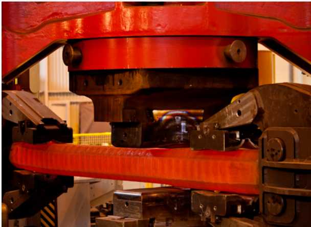
UKAD state-of-the-art facility with 4,500 ton forging press and lean manufacturing environment
