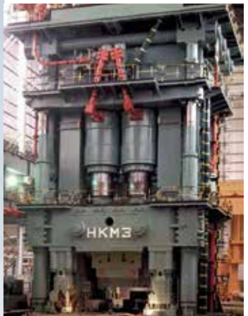
65,000 tons closed-die forging press
