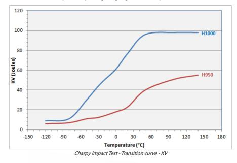
510°C (H950): this aging condition is used for high strength requirements such as aircraft structural parts
