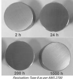
Passivation: Type 8 as per AMS 2700 Salt spray test as per ASTM B117
