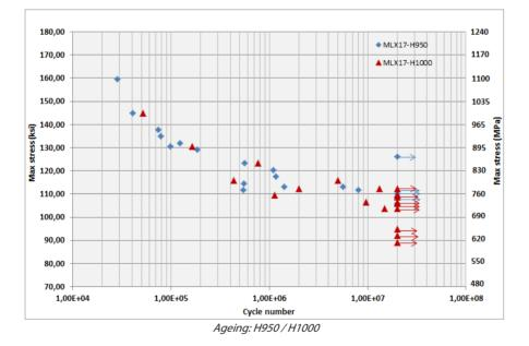
Fatigue performance of MLX<sup>®</sup>17 is equivalent to Custom465<sup>®</sup>. Typical failure initiation is at a cleavage zone or starts at a Ti-C-N particle or both. This behavior is typical of any Ultra High Strength maraging steels hardened with a high amount of titanium and/or aluminum.
