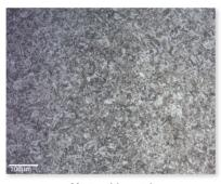
Martensitic matrix (optical microscopy)
