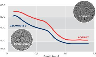
Comparison of hardness profil between AD65N™ and 33CrMoV12-9 grade after deep nitriding (Nitriding temperature: ≈ 550°C - Duration : ≈ 120 hours.)
