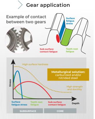
There are three main types of stress that occur when two gears come into contact:
