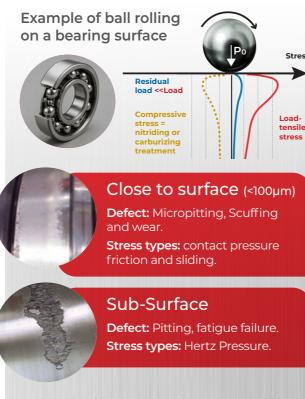
The loading of a ball in contact with a raceway provides tensile stresses that can be compensated by increasing the surface hardness and introducing of the compressive stresses.
