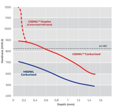
Comparison of hardness profil between M50NIL and C65NIL<sup>™</sup> grade after carburizing
