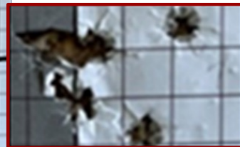
Yaw measurements indicate barrel has reached failure level for MIL-B-11595.
