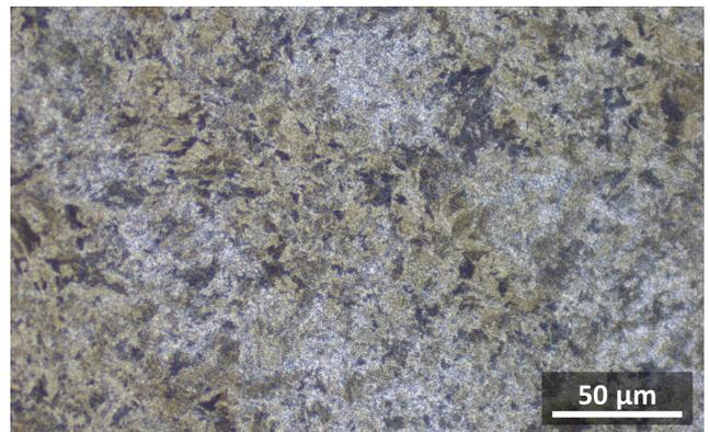
Microstructure after heat treatment at 845°C/30min/Air + 610°C/4h giving a hardness of 44.5 HRC
