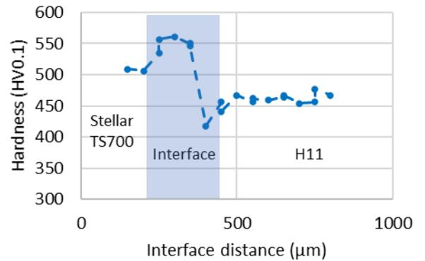
Hardness of the interface between Stellar TS700 to H11 as-printed
