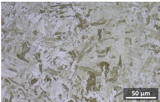
Microstructure after heat treatment at 1090°C + 680°C/4h giving a hardness of 48 HRC.
