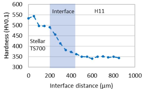
Hardness of the interface between Stellar TS700 to H11 after aging at 650°C
