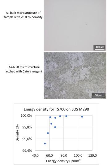
Density measured by optical method
