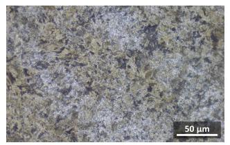
Microstructure after heat treatment at 845°C/30min/Air + 610°C/4h giving a hardness of 44.5 HRC
