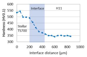
Hardness of the interface between Stellar TS700 to H11 after aging at 650°C
