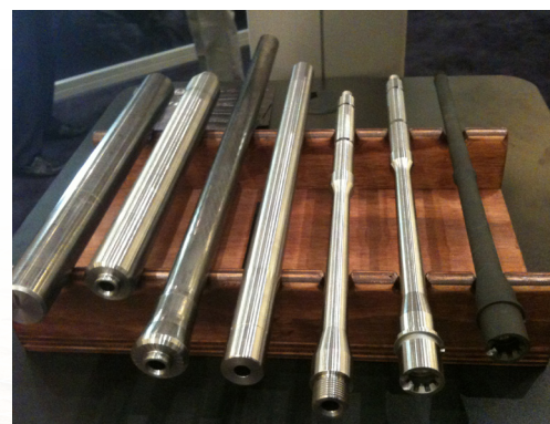
Gun Barrel Shape Evolution during the Forming Process
