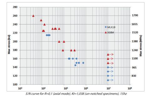
Fatigue performance of MLX®19 is lower than 300M. Typical failure initiation is at a cleavage zone or starts at a Ti-C-N particle or both. This behavior is typical of any Ultra High Strength maraging steels hardened with a high amount of titanium and/or aluminum.
