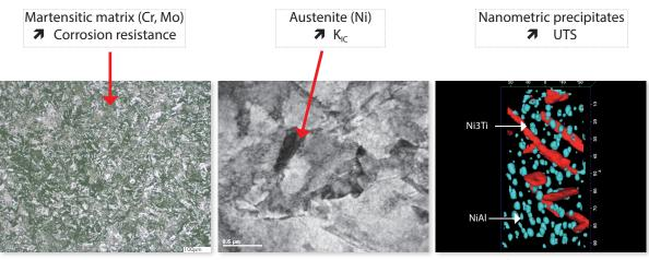
Martensitic matrix (optical microscopy)
