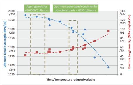
Combination of Ultimate Tensile Strength and Fracture Thoughness  $K_{LC}$
