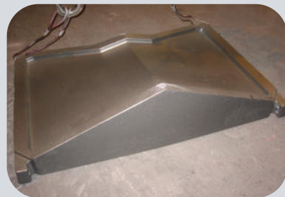
Tooling for Jet flap or windshield front fairing of airplane
