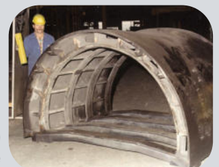
Tooling for A380 engine nacelle
